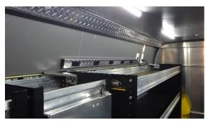
There are two lengths of the Superstrut on each side of the equipment area, one high and one low, to facilitate even distribution of weight on the attachment points. Electrical outlets, both 110 and 12 volts, were installed high on both the driver and passenger side of the tool area above the shelving. This allowed the installation of RPT's on each side to accommodate all equipment battery chargers.
